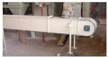
The round return end of the chain conveyor is equipped with 10 mm Nonfric in the outer surface.
