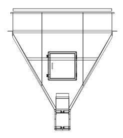
Intake pit, built on top of chain conveyor with intermediate bottom. The side wall of the intake pit is designed with a 60° slope and is very suitable for difficult products, such as meat and bone meal, fish meal and similar products that tend to bridging in the intake pit.
