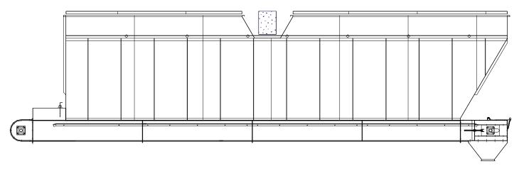
Bin scale built similar to the intake pit above. The intermediate bottom is in full length of the bin, and is avoiding the products to be bridging.
