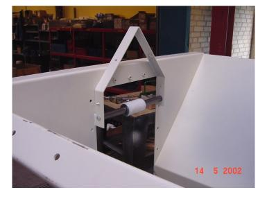
Details in the end of the side inlet section, where the bracket for the top cover is seen, and the return roller as well.
