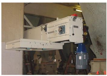
The combined tension and drive section is standard in the A 40 S to A 800 S chain conveyor.
