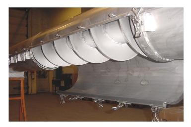
The screw blades are manufactured from heavy steel.
