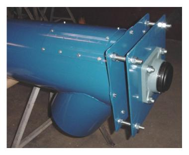
The FM tube screw conveyors are often equipped with ROTOGLYD sealings.
