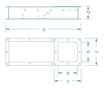
This simple hand-operated shutter is mainly used for security- / repair- shutters, and can also be used for silo outlets.
