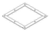
Assembly for 300 and 400 mm are always done with bolted flanges – which also are available for 160 – 200 and 240 mm sizes.
