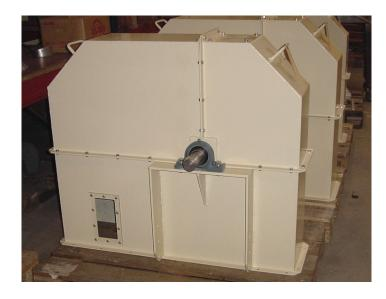
The elevator head is provided with pedestal bearings, which are a very stabile and strong structure, enabling dismantling both top cover parts for service and maintenance.
